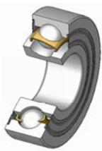
Angular contact ball bearings use axially asymmetric races. The raceways in the inner and outer rings have a raised shoulder which is displaced with respect to each other in the direction of the bearing axis.<sup>30</sup> (See Angular Contact Ball Bearing photo to the left; *provided courtesy of Wikipedia*). In simpler terms, this means that these bearings are designed to accommodate combined loads (loads in both the radial and axial directions).
